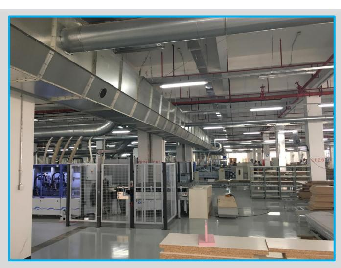
Beside optimized flexibility and reduced energy cost, the Multiflow channel functions as a pre-filter, where up to 80% of the exhausted dust is separated in the channel. Only very fine dust escapes to the dust collector, which reduces the wear and tear on the filter system and increase the life span of filter bags by up to 2 years.
