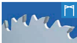
ATB Alternate top bevel teeth positive with chip limiter (=WZ pos.)
