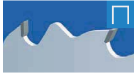
Flat with chip limiter (=FZ)
