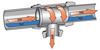
This fitting is also an alternative to a traditional goose neck (up and over) take-off point. It prevents water from dropping out of the main piping loop into the drop line. All systems should be installed with a slight gradient to allow moisture to collect at one point in the system. This point should be fitted with a drop line and terminated with a condensate drain.
